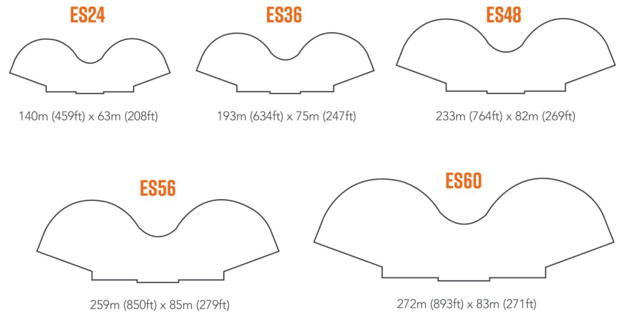
*ES24 through ES60 are primary sizings, although we can accommodate lagoons larger and smaller or with any number of caissons in between.*
